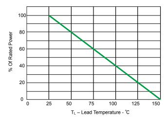
Fig 2.Power Derating Curve
