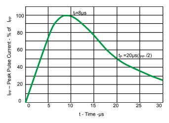
Fig 1.Pulse Waveform
