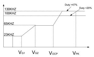
As the output load current is decreased, the IC enter into green mode smoothly from the PWM mode. In this mode, the switching frequency will start to linearly decrease from 65KHz to 23KHz, meanwhile the valley turn on can be realized by monitoring the voltage activity on auxiliary windings through the PRT pin. So the switching loss is minimized and the high conversion efficiency can be achieved.
