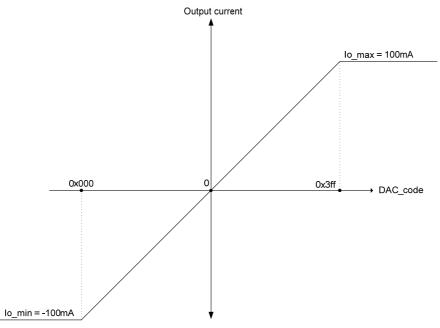
Figure 6. Description of Output Current Characteristics
