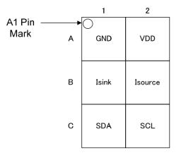
Figure 2. Pin Configuration (Top View)
