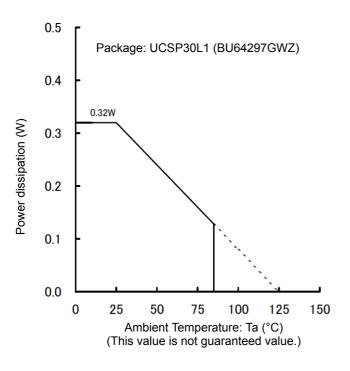
Figure 7. Power dissipation Pd [W]
