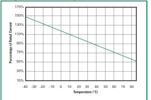
Note: The average time current curves and Temperature Rerating curve performance is affected
