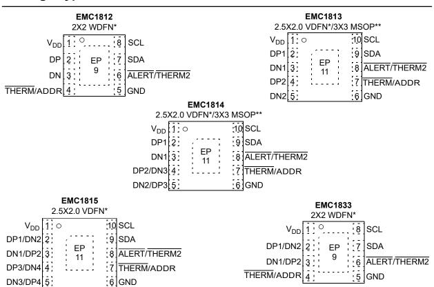
Note: \*Includes Exposed Thermal Pad (EP). See Section 3. Pin Descriptions.
