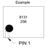
10-Lead MSOP (3 x 3 mm)
