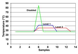
The filter consists of a running average on the external diode channel. The Level 1 filter is a running average of 4x while the Level 2 filter is a running average of 8x. For the first measurement immediately after power-up, the filter will be filled with the results of the first measurement. After this, the filter is operated normally. Any temperature comparisons are done with the filtered results that are stored in the user register.
