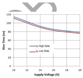
Figure 9. Rise Time vs. Supply Voltage
