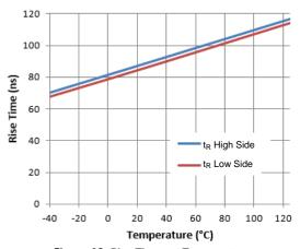
Figure 10. Rise Time vs. Temperature
