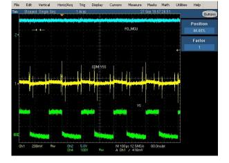
**Figure 35.** During startup current is high, with cap between COM-VSS, noise is less, fault conditions do not occur, compressor will not stall, 100us/div
