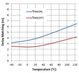
Figure 16. Delay Matching vs. Temperature
