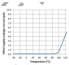
Figure 26. Offset Supply Leakage Current vs. Temperature
