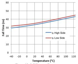
Figure 12. Fall Time vs. Temperature
