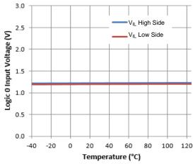
Figure 24. Logic 0 Input Voltage vs. Temperature
