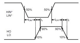
Figure 1. Switching Time Waveform Definitions
