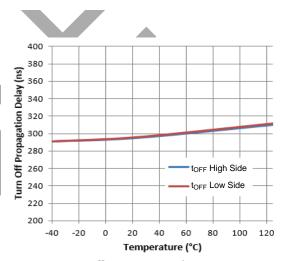
Figure 8. Turn-off Propagation Delay vs. Temperature
