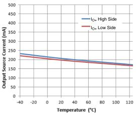
Figure 18. Output Source Current vs. Temperature
