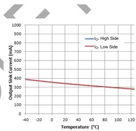
Figure 20. Output Sink Current vs. Temperature
