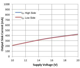
Figure 19. Output Sink Current vs. Supply Voltage
