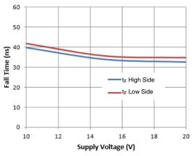
Figure 11. Fall Time vs. Supply Voltage
