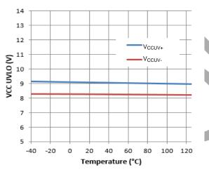
Figure 25. VCC UVLO vs. Temperature
