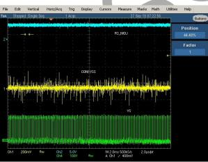
**Figure 34.** During startup current is high, with cap between COM-VSS, noise is less, fault conditions do not occur, compressor will not stall, 2ms/div
