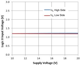
Figure 23. Logic O Input Voltage vs. Supply Voltage
