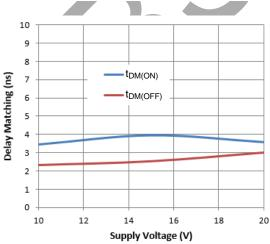
Figure 15. Delay Matching vs. Supply Voltage
