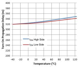
Figure 6. Turn-on Propagation Delay vs. Temperature
