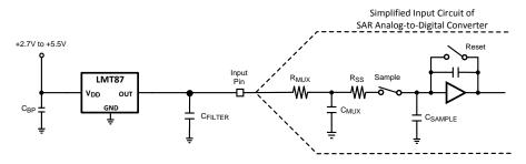
Figure 13. Suggested Connection to a Sampling Analog-to-Digital Converter Input Stage
