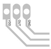
Figure 21. TO-92 LP Package Recommended Layout
