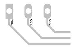
Figure 22. TO-92 LPM Package Recommended Layout
