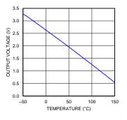
Figure 14. Analog Output Transfer Function
