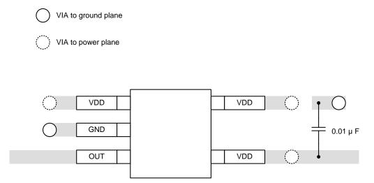
Figure 20. SC70 Package Recommended Layout
