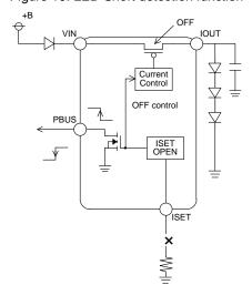
Figure 20. ISET Pin open detection function
