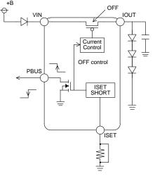
Figure 21. ISET Pin short detection function
