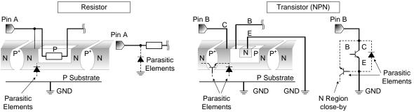
Figure 26. Example of monolithic IC structure
