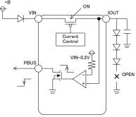
Figure 18. LED Open detection function
