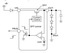
Figure 19. LED Short detection function
