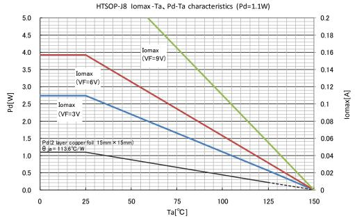
Figure 25. Heat reduction curve
