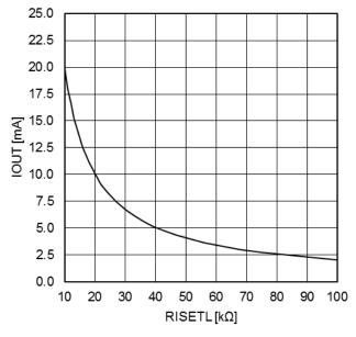
Figure 5.  $I_{OUT}$  vs  $R_{ISETL}$  (STOP=Low)
