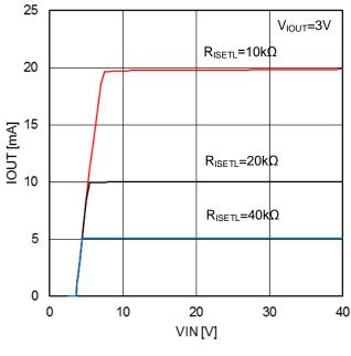
Figure 7.  $I_{OUT}$  vs  $V_{IN}$  (STOP=Low)
