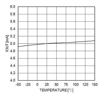
Figure 9. I<sub>OUT</sub> vs Ta (STOP=Low)
