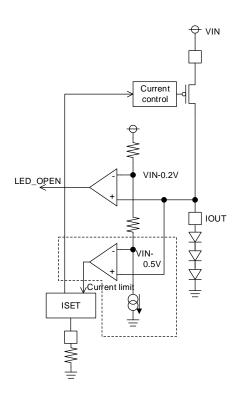
Figure 15. Current Control at Output Saturation
