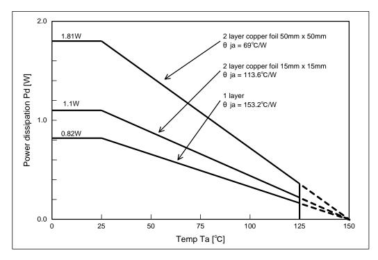
(Caution1) When mounted with 70.0mm x 70.0mm x 1.6mm glass epoxy substrate.
