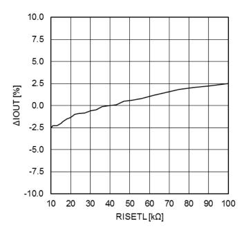
Figure 11.  $\Delta I_{OUT}$  vs  $R_{ISETL}$  (STOP=Low)
