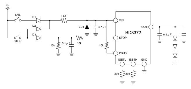
Figure 23. Recommended application circuit
