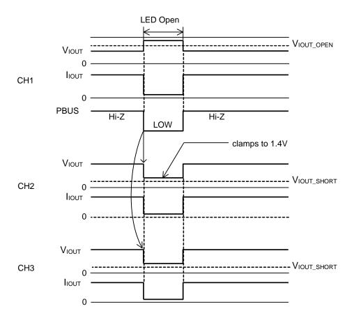
Figure 17. Example of protective Operation
