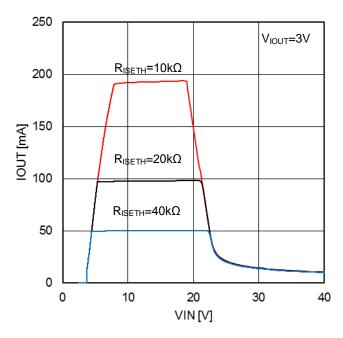
Figure 8. I<sub>OUT</sub> vs V<sub>IN</sub> (STOP=High)
