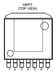
Figure 2. HRP7 Package Pin Configuration
