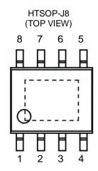
Figure 3. HTSOP-J8 Package Pin Configuration
