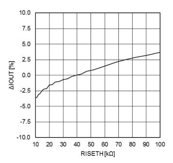
Figure 12.  $\Delta I_{OUT}$  vs R<sub>ISETH</sub> (STOP=High)
