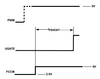
FIGURE 3. PS4 EXIT TIMING DIAGRAM
