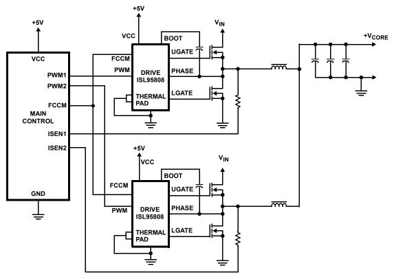
FIGURE 2. TYPICAL APPLICATION WITH 2-PHASE CONVERTER
