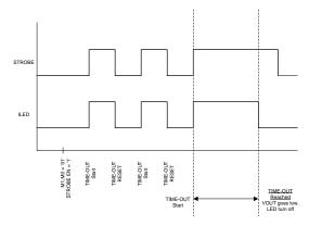
(1) When the flash timer elapses, the device goes into stand-by regardless of strobe state
