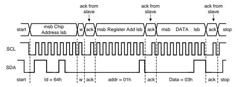
Figure 22. Write Cycle W = Write (SDA = 0) R = Read (SDA = 1) Ack = Acknowledge (SDA Pulled Down by Either Master or Slave) ID = Chip Address, 64h for LM36011
