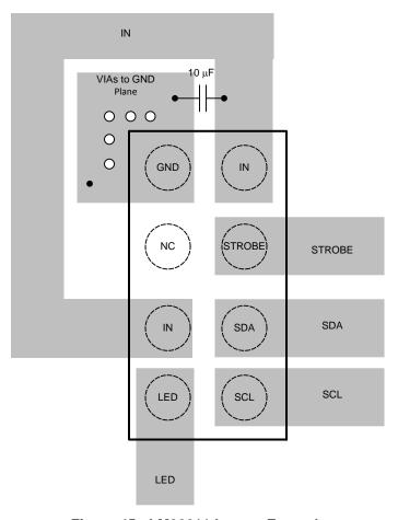
Figure 45. LM36011 Layout Example
