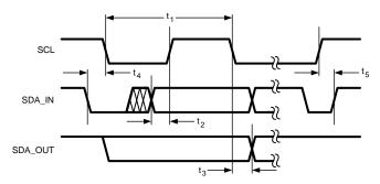
Figure 1. I<sup>2</sup>C-Compatible Interface Specifications
