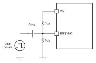
Figure 7-5. Synchronizing to External Clock
