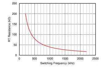
Figure 7-2. RT vs Frequency Curve
