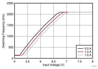
Figure 7-8. Frequency Foldback at Dropout (V<sub>OUT</sub> = 5 V, f<sub>SW</sub> = 2100 kHz)
