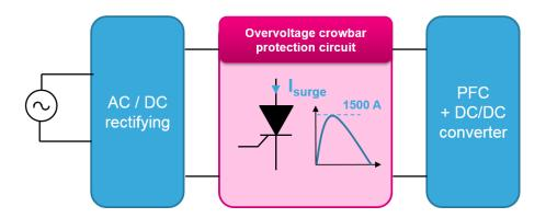
In case of overvoltage on line power terminals (example: lightning event), the voltage is rising quickly across the DC/DC module and can reach voltages limitations of devices, leading to possible application failure. The overvoltage crowbar protection answers to this issue by placing the SCR in parallel of the rectifier bridge output, and limiting the induced surge current during electrical over-stress.
