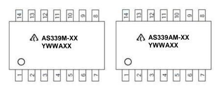
First Line: Logo and Marking ID (See Ordering Information) Second Line: Date Code Y: Year WW: Work Week of Molding A: Assembly House Code XX: 7<sup>th</sup> and 8<sup>th</sup> Digits of Batch Number
