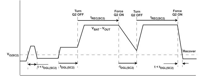
Figure 24. OUT Short-Circuit – Supplement Mode
