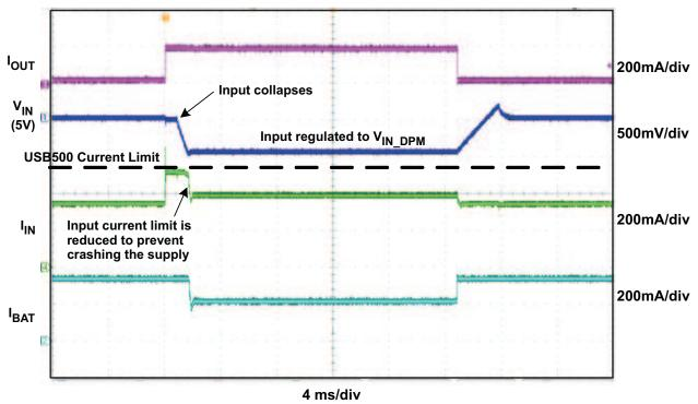
Figure 15. V<sub>IN</sub>-DPM Waveform
