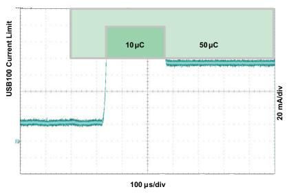
Figure 14. USB-IF Inrush Current Test
