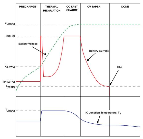
Figure 19. Charge Cycle Modified by Thermal Loop
