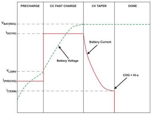
Figure 17. Typical Charge Cycle
