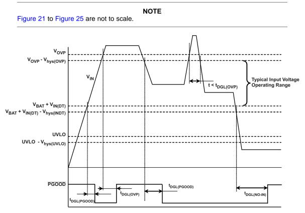
Figure 21. Power-Up, Power-Down, Power Good Indication
