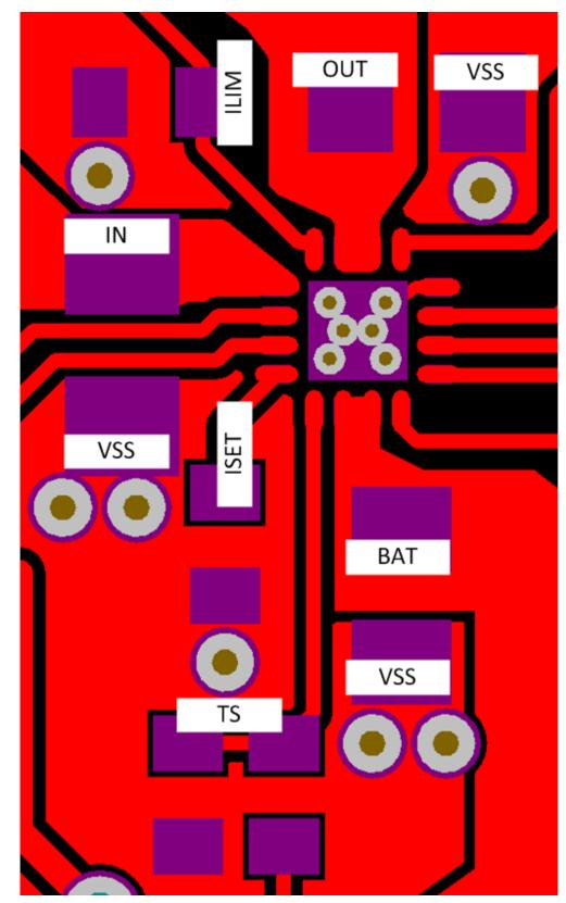
Figure 37. Layout Schematic
