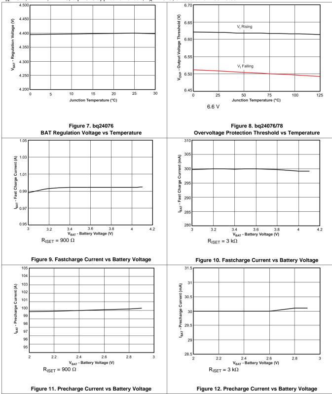
$V_{IN}$  = 6 V, EN1=1, EN2=0, bq24078 application circuit,  $T_A$  = 25°C, unless otherwise noted.
