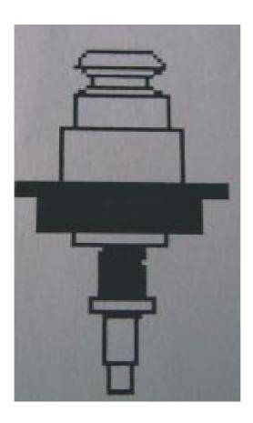
dimension of nozzle:504 external diameter: 1.5mm; inside diameter: 1.0mm;
