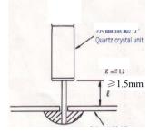
(2)當用手工來彎曲引線時,請遵照下列方法When the lead needs to be bent by hand, please follow the instruction as below: 用手指捏住圓柱晶體的外殼;用鑷子夾住引線要彎曲的部位,該部位離晶體基座底部1.5mm以上(推薦3.0mm); 用鑷子夾住彎曲引線成90°,不要用力拉引線。用力拉引線可能造成引線根部的玻璃子破裂,而産生漏氣損壞元件電性能。 Hold the body of the cylinder type crystal unit in fingers;
