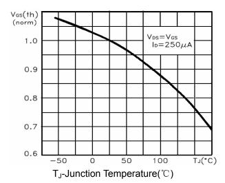
Figure 10 V<sub>GS(th)</sub> vs Junction Temperature
