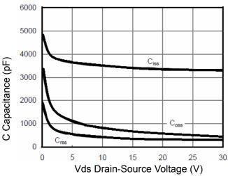
Figure 7 Capacitance vs Vds
