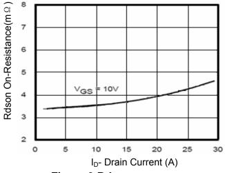
Figure 3 Rdson- Drain Current
