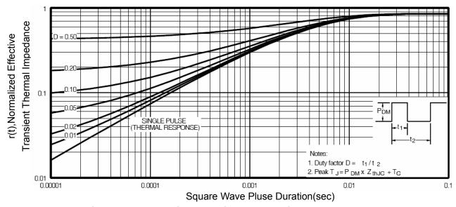
**Figure 11 Normalized Maximum Transient Thermal Impedance**
