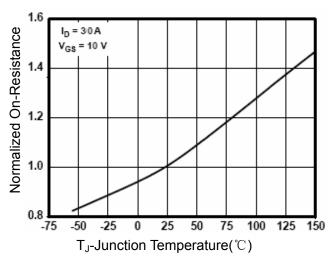
Figure 4 Rdson-JunctionTemperature
