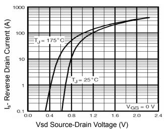
Figure 6 Source- Drain Diode Forward
