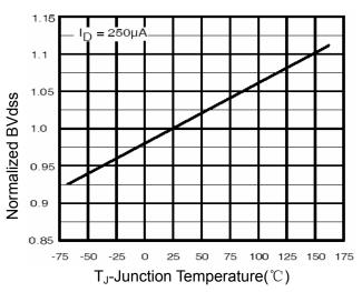
Figure 9 BV<sub>DSS</sub> vs Junction Temperature
