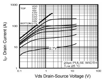
**Figure 1 Output Characteristics**
