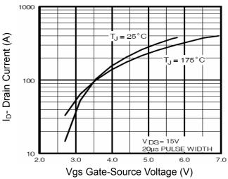
**Figure 2 Transfer Characteristics**
