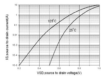
Figure 4 Body diode Characteristics
