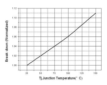
Figure 6 BVDSS vs Junction Temperature
