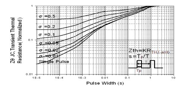
**Figure 11 Normalized Maximum Transient Thermal Impedance**
