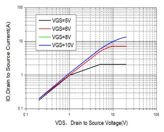
**Figure 1 Output Characteristics**
