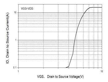
**Figure 2 Transfer Characteristics**
