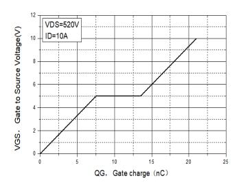
Figure 8 VGS vs QG Characteristics
