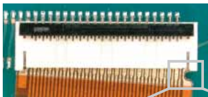
Incomplete FPC insertion
