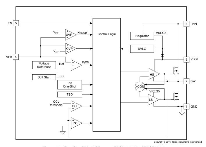
Figure 19. Functional Block Diagram: TPS562200 And TPS563200
