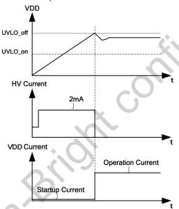
Fig1 Startup current timing
