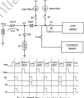
Fig4 PRT Pin protection timing
