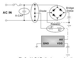
Fig9 X-CAP discharge circuit
