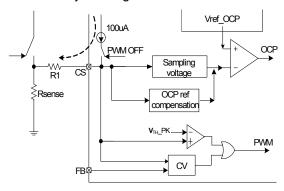
Fig.5 Programmable OCP and PK load protection
