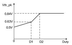
Fig6 Cycle by cycle OCP compensation
