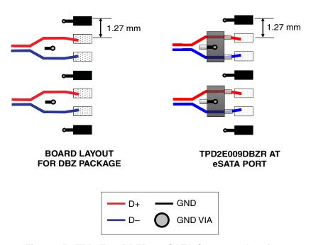
Figure 15. TPD2E009DBZR at eSATA Connector Interface
