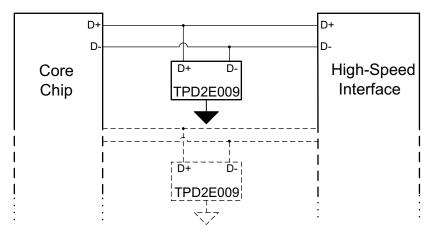
Figure 7. TPD2E009 in a High-Speed Interface
