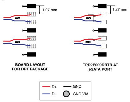
Figure 14. TPD2E009DRTR at eSATA Connector Interface
