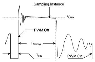
Figure.2. Auxiliary voltage waveform
