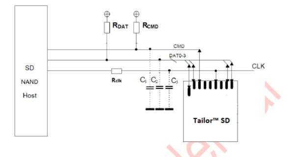
RDAT and RCMD (10K~100 k $\Omega$ ) are pull-up resistors protecting the CMD and the DAT lines against bus floating when Nano SD NAND is in a high-impedance mode.
