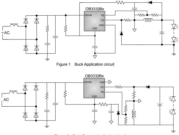
Figure 2 Buck-Boost Application circuit
