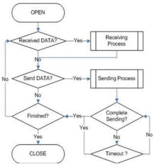
Fig 15. IPRAW Operation Flow
