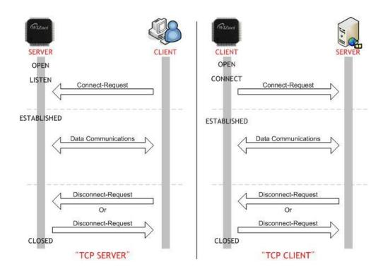
Fig 9. "TCP SERVER" & "TCP CLIENT"
