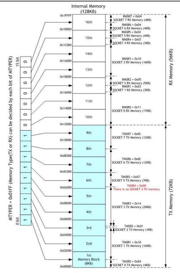
Fig 8. Allocation Internal TX/RX memory of SOCKETn
