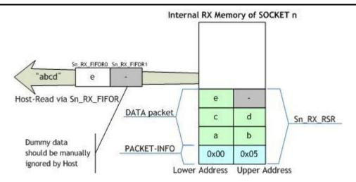
Fig 7. Access to Internal RX Memory
