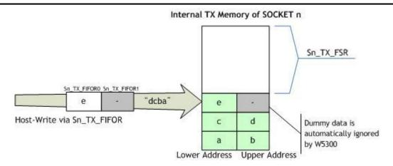
Fig 6. Access to Internal TX Memory
