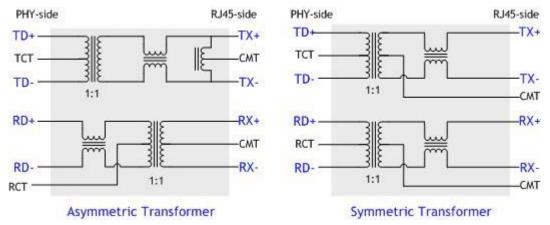
In case of using internal PHY mode, be sure to use symmetric transformer in order to support Auto MDI/MDIX(Crossover).
