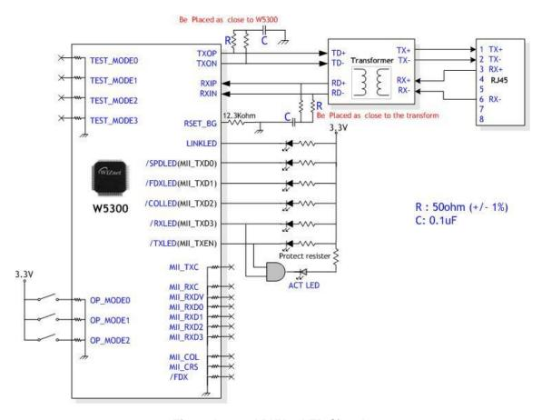
Fig 19. Internal PHY & LED Signals
