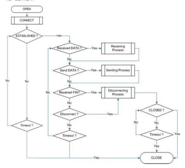
Fig 12. "TCP CLIENT" Operation Flow
