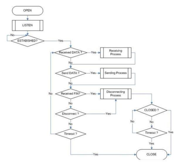
Fig 10. "TCP SERVER" Operation Flow
