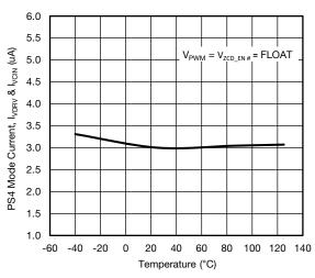
Fig. 17 - PS4 Mode Current vs. Temperature
