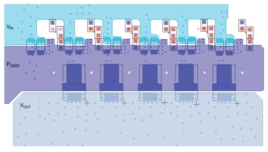
Fig. 19 - Multi - Phase VRPower Layout Bottom View
