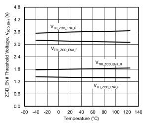
Fig. 16 - ZCD\_EN# Threshold vs. Temperature
