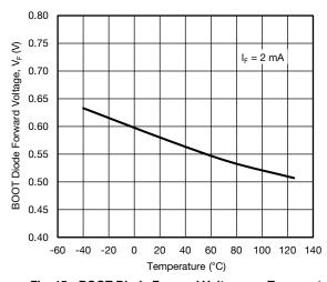
Fig. 15 - BOOT Diode Forward Voltage vs. Temperature
