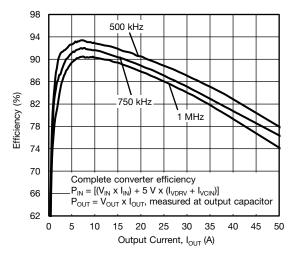
Fig. 8 - Efficiency vs. Output Current ( $V_{IN} = 9 V$ )
