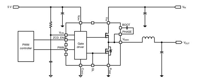
Fig. 1 - SiC631 Typical Application Diagram
