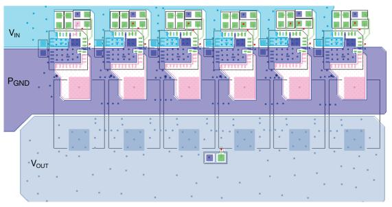
Fig. 18 - Multi - Phase VRPower Layout Top View
