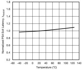
Fig. 14 - PS4 Exit Latency vs. Temperature
