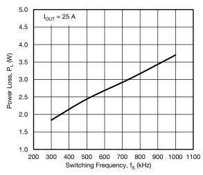
Fig. 7 - Power Loss vs. Switching Frequency (V<sub>IN</sub> = 12.6 V)
