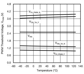
Fig. 13 - PWM Threshold vs. Temperature
