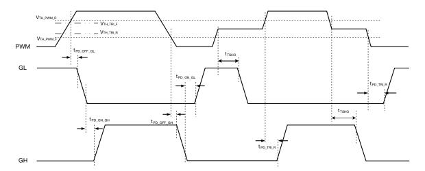
Fig. 4 - Definition of PWM Logic and Tri-state
