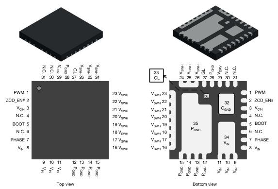
Fig. 2 - SiC631 Pin Configuration
