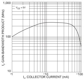
Figure 3 Gain-Bandwidth Product vs Collector Current
