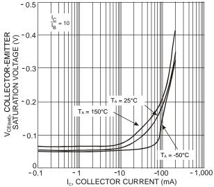
Figure 2 Typical Collector-Emitter Saturation Voltage vs. Collector Current
