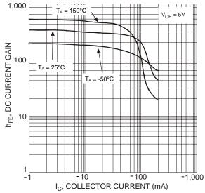
Figure 1 Typical DC Current Gain vs. Collector Current
