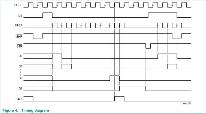
8-bit shift register with output register
