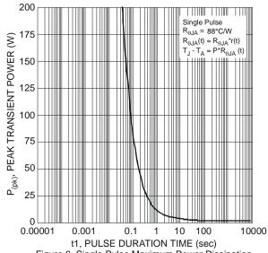
Figure 6 Single Pulse Maximum Power Dissipation
