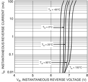
V<sub>R</sub>, INSTANTANEOUS REVERSE VOLTAGE (V) Fig. 3 Typical Breakdown Characteristics
