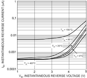
V<sub>R</sub>, INSTANTANEOUS REVERSE VOLTAGE (V) Fig. 4 Typical Low Current Reverse Characteristics
