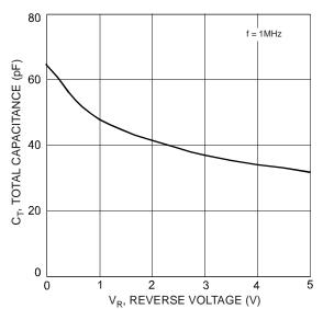
Fig. 5 Typical Total Capacitance vs. Reverse Voltage
