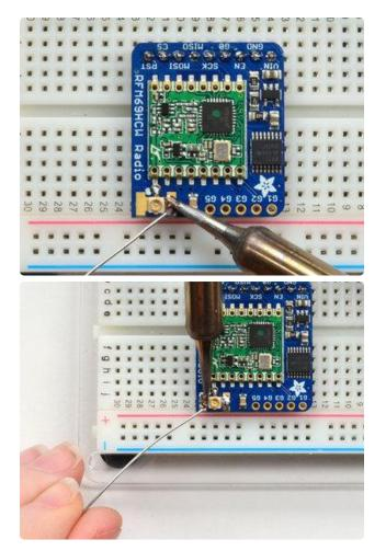
Solder in the two side pads, they are used for signal and mechanical connectivity so make sure there's plenty of solder
