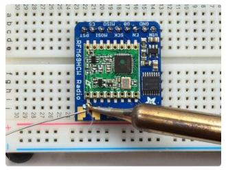
Put down a touch of solder on the signal pad
