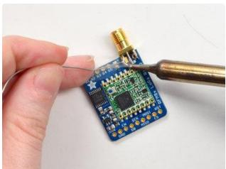
Solder in the two side ground pads. Note you will need a lot of heat for this, because the connector is an excellent heat sink and its got a huge ground plane
