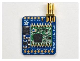
The SMA connector 'slides on' the top of the PCB
