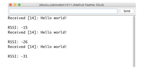
To receive a message simply call the <a href="receive">receive</a> function. This function will wait for half a second for any packet to be received. If a packet is found it will be returned as
