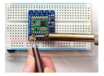
Solder in the first pad while holding the uFL steady
