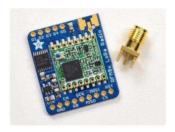
You'll need an SMA (or, if you need RP-SMA for some reason) Edge-Mount connector with 1.6mm spacing
