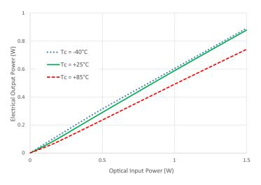
Figure 8: Typical Output Voltage vs. Optical Input Power of AFBR-POCx06L at Different Case Temperatures
