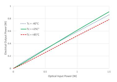
Figure 5: Typical Output Voltage vs. Optical Input Power of AFBR-POCx04L at Different Case Temperatures
