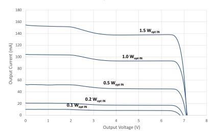
Figure 7: Typical Electrical Output Power vs. Optical Input Power of AFBR-POCx06L at Different Case Temperatures
