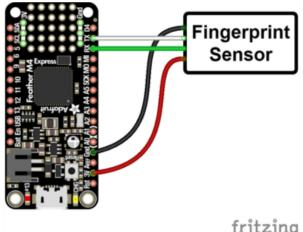
Board GND to sensor GND (black wire) Board TX to sensor RX (white wire) Board RX to sensor TX (green wire) Board 3.3v to sensor VCC (red wire)
