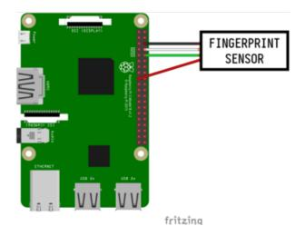
Pi GND to sensor GND (black wire) Pi TX to sensor RX (white wire) Pi RX to sensor TX (green wire) Pi 3.3v to sensor VCC (red wire)
