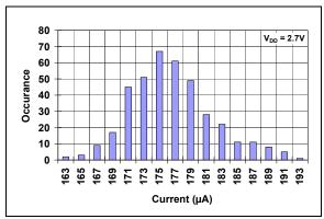
FIGURE 2-13: I<sub>DD</sub> Histogram.
