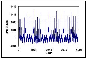
FIGURE 2-1: DNL vs. Code  $(V_{DD} = 5.5V)$ .
