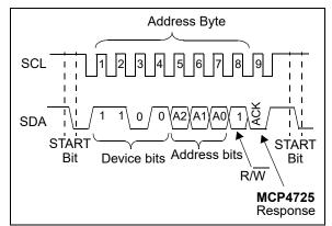
FIGURE 8-2: I<sup>2</sup>C Bus Connection Test.
