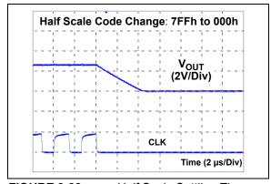
FIGURE 2-22: Half Scale Settling Time.
