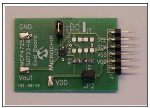
FIGURE 9-1: MCP4725 SOT-23-6 Evaluation Board.
