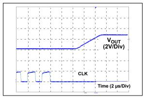
FIGURE 2-24: Exiting Power Down Mode.
