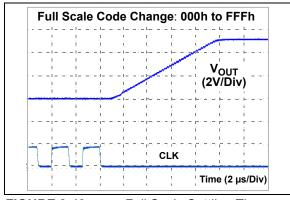
FIGURE 2-19: Full Scale Settling Time.
