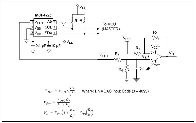
**EXAMPLE 8-3:** Digitally-Controlled Bipolar Voltage Source.
