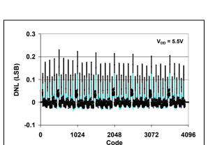
**FIGURE 2-2:** DNL vs. Code and Temperature ( $T_A = -40^{\circ}\text{C}$  to +125°C).
