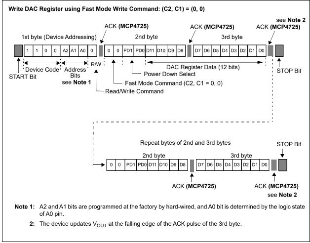
FIGURE 6-1: Fast Mode Write Command.
