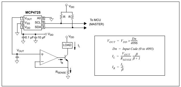
FIGURE 8-3: Digitally Controllable Current Source.
