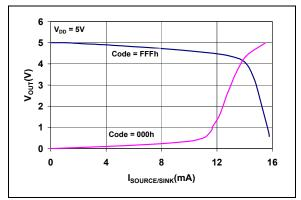
FIGURE 2-16: Source and Sink Current Capability.
