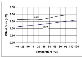
**FIGURE 2-14:** Offset Error vs. Temperature and  $V_{DD}$ .
