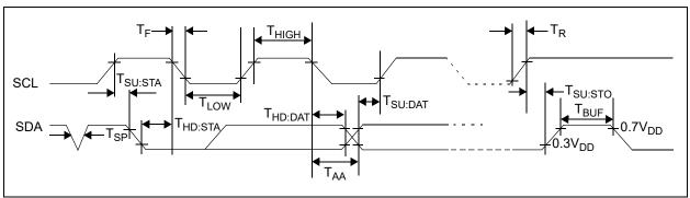
FIGURE 7-4: I<sup>2</sup>C Bus Timing Data.
