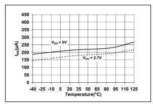
FIGURE 2-11: I<sub>DD</sub> vs. Temperature.
