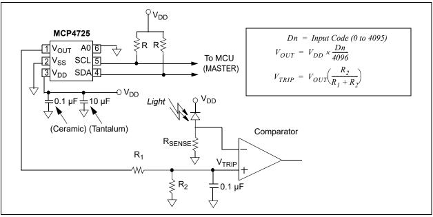
**EXAMPLE 8-1:** Set Point Or Threshold Calibration.
