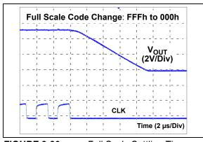
FIGURE 2-20: Full Scale Settling Time.
