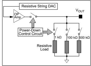
FIGURE 5-1: Output Stage for Power-Down Mode.
