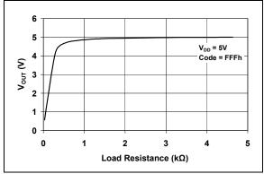
FIGURE 2-15: V<sub>OUT</sub> vs. Resistive Load.
