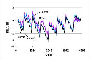
**FIGURE 2-6:** INL vs. Code and Temperature  $(V_{DD} = 5.5V)$ .
