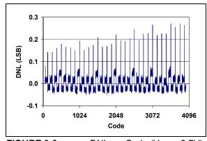
FIGURE 2-3: DNL vs. Code  $(V_{DD} = 2.7V)$ .
