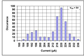
FIGURE 2-12: I<sub>DD</sub> Histogram.
