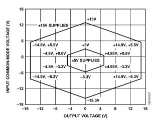
Figure 27. Input Common-Mode Voltage Range vs. Output Voltage, G = 1,  $V_{REF} = 0$  V
