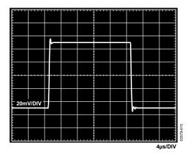
Figure 50. Small Signal Pulse Response, G=10,  $R_{LOAD}=2$   $k\Omega$ ,  $C_{LOAD}=100$  pF,  $V_S=5$  V,  $V_{REF}=2.5$  V
