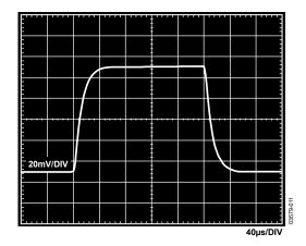
Figure 52. Small Signal Pulse Response, G=1000,  $R_{LOAD}=2$   $k\Omega$ ,  $C_{LOAD}=100$  pF,  $V_{S}=5$  V,  $V_{REF}=2.5$  V
