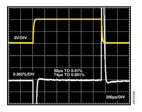
Figure 44. Large Signal Pulse Response and Settle Time, G = 1000,  $R_{LOAD}=10~k\Omega,~V_S=\pm15~V,~V_{REF}=0~V$
