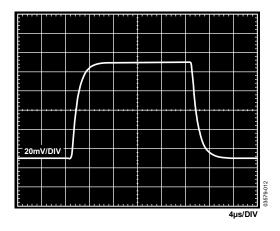
Figure 47. Small Signal Pulse Response, G=100,  $R_{LOAD}=2$  k $\Omega$ ,  $C_{LOAD}=100$  pF,  $V_S=\pm15$  V,  $V_{REF}=0$  V
