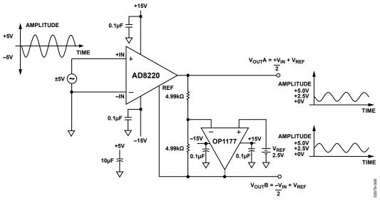
Figure 65. Differential Output with Level Shift
