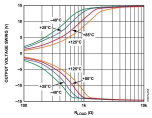
Figure 34. Output Voltage Swing vs. Load Resistance  $V_S = \pm 15 \text{ V}$ ,  $V_{REF} = 0 \text{ V}$
