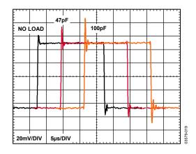
Figure 39. Small Signal Pulse Response for Various Capacitive Loads,  $V_S = 5 V$ ,  $V_{REF} = 2.5 V$
