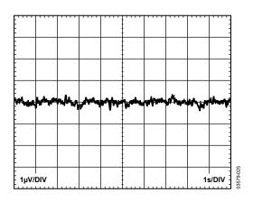
*Figure 12. 0.1 Hz to 10 Hz RTI Voltage Noise (G* = 1000)
