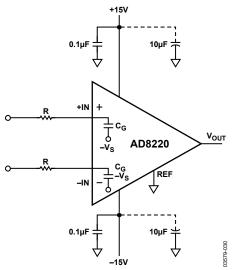
Figure 61. RFI Filtering Without External Capacitors
