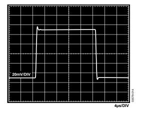
Figure 46. Small Signal Pulse Response, G=10,  $R_{LOAD}=2$   $k\Omega$ ,  $C_{LOAD}=100$  pF,  $V_S=\pm 15$  V,  $V_{REF}=0$  V
