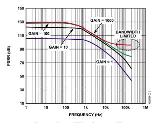
Figure 14. Positive PSRR vs. Frequency, RTI
