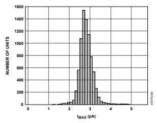
Figure 8. Typical Distribution of Input Bias Current
