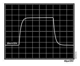
Figure 48. Small Signal Pulse Response, G=1000,  $R_{LOAD}=2~k\Omega$ ,  $C_{LOAD}=100~pF,~V_S=\pm15~V,~V_{REF}=0~V$
