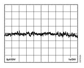
Figure 11. 0.1 Hz to 10 Hz RTI Voltage Noise (G = 1)
