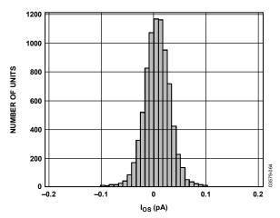
Figure 9. Typical Distribution of Input Offset Current
