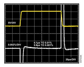
Figure 43. Large Signal Pulse Response and Settle Time, G=100,  $R_{LOAD}=10~k\Omega,~V_S=\pm15~V,~V_{REF}=0~V$
