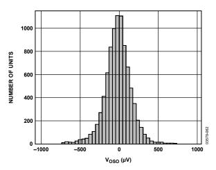
Figure 7. Typical Distribution of Output Offset Voltage
