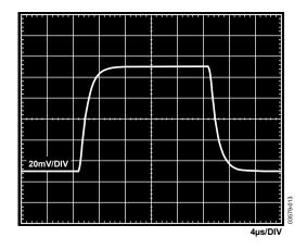
Figure 51. Small Signal Pulse Response, G=100,  $R_{LOAD}=2$  k $\Omega$ ,  $C_{LOAD}=100$  pF,  $V_S=5$  V,  $V_{REF}=2.5$  V
