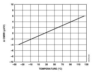
Figure 21. Change in CMRR vs. Temperature, G = 1
