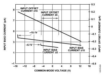
Figure 16. Input Bias Current and Input Offset Current vs. Common-Mode Voltage
