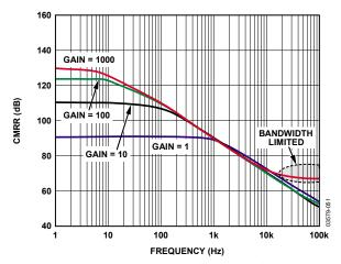
Figure 20. CMRR vs. Frequency, 1 k $\Omega$  Source Imbalance
