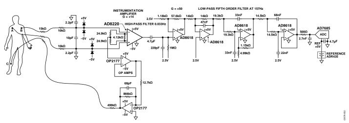
Figure 67. Example ECG Schematic
