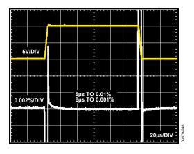
Figure 41. Large Signal Pulse Response and Settle Time, G=1,  $R_{LOAD}=10~k\Omega,~V_S=\pm15~V,~V_{REF}=0~V$
