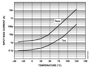
Figure 17. Input Bias Current and Offset Current vs. Temperature,  $V_S=\pm 15~V, V_{\it REF}=0~V$
