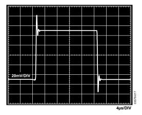
Figure 49. Small Signal Pulse Response, G=1,  $R_{LOAD}=2$  k $\Omega$ ,  $C_{LOAD}=100$  pF,  $V_S=5$  V,  $V_{REF}=2.5$  V
