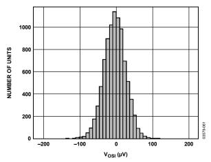
Figure 6. Typical Distribution of Input Offset Voltage
