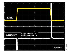
Figure 42. Large Signal Pulse Response and Settle Time, G=10,  $R_{LOAD}=10~k\Omega$ ,  $V_S=\pm15~V$ ,  $V_{REF}=0~V$
