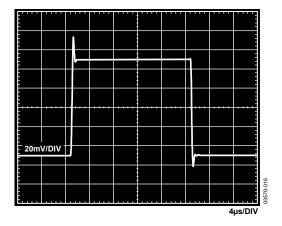
Figure 45. Small Signal Pulse Response, G=1,  $R_{LOAD}=2$   $k\Omega$ ,  $C_{LOAD}=100$  pF,  $V_S=\pm 15$  V,  $V_{REF}=0$  V
