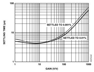
Figure 54. Settling Time vs. Gain for a 10 V Step,  $V_S = \pm 15 \text{ V}$ ,  $V_{REF} = 0 \text{ V}$
