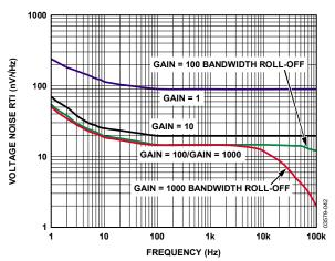
Figure 10. Voltage Spectral Density vs. Frequency
