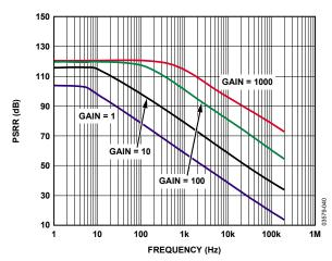
Figure 15. Negative PSRR vs. Frequency, RTI
