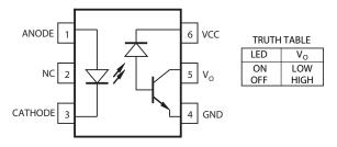
A 0.1  $\mu F$  bypass capacitor between pins 4 and 6 is recommended.
