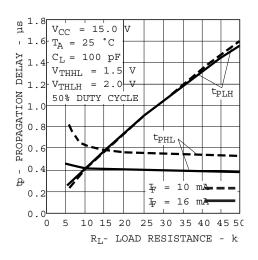
Figure 9 Propagation Delay Time vs. Load Resistance
