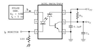
Figure 7 Test Circuit for Transient Immunity and Typical Waveforms
