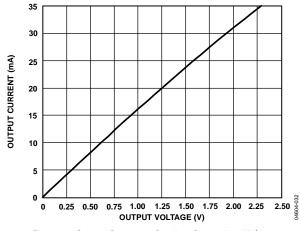
Figure 23. Output Current vs. Receiver Output Low Voltage
