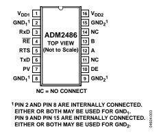
Figure 2. Pin Configuration
