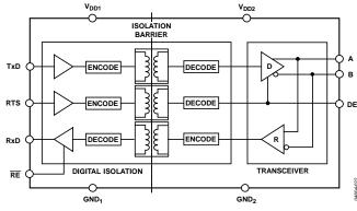
Figure 26. ADM2486 Digital Isolation and Transceiver Sections
