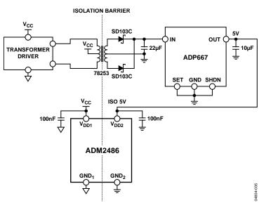
Figure 32. Isolated Power Supply Circuit
