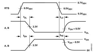
Figure 14. Driver Enable/Disable Timing
