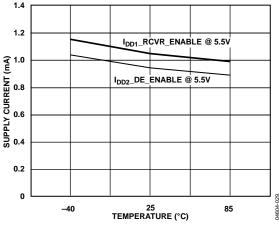
Figure 16. Unloaded Supply Current vs. Temperature
