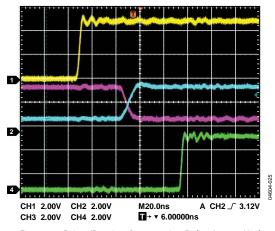
Figure 19. Driver/Receiver Propagation Delay, Low to High  $(R_{LDiff} = 54 \ \Omega, C_{L1} = C_{L2} = 100 \ pF)$
