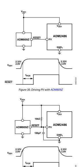
Figure 31. Driving PV with an Open-Drain Output
