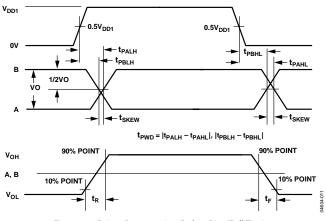
Figure 12. Driver Propagation Delay, Rise/Fall Timing
