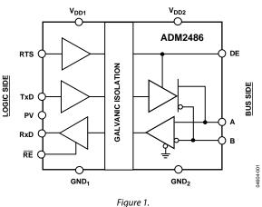
The ADM2486 driver has an active-high enable feature. The driver differential outputs and the receiver differential inputs are connected internally to form a differential input/output port that imposes minimal loading on the bus when the driver is disabled or when VDD1 or VDD2 = 0 V. Also provided is an active-high receiver disable feature that causes the receive output to enter a high impedance state.
