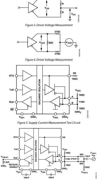
Figure 6. High Frequency Common-Mode Noise Test Circuit
