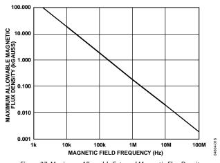
Figure 27. Maximum Allowable External Magnetic Flux Density
