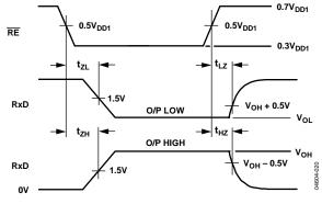
*Figure 15. Receiver Enable/Disable Timing*
