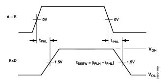
Figure 13. Receiver Propagation Delay
