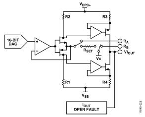
Figure 74. Voltage to Current Conversion Circuitry
