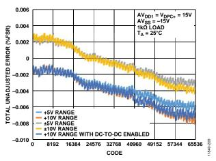
Figure 9. Total Unadjusted Error vs. DAC Code
