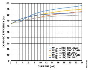
Figure 57. DC-to-DC Efficiency vs. Current
