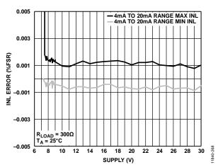
Figure 48. INL Error vs. AVDD1/AVss Supply, External RSET
