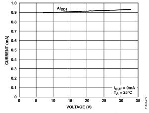
Figure 71. Al<sub>DD1</sub> Current vs AV<sub>DD1</sub> Supply
