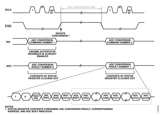
Figure 85. ADC Conversion Timing Example
