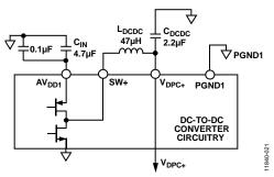
Figure 77. DC-to-DC Circuit
