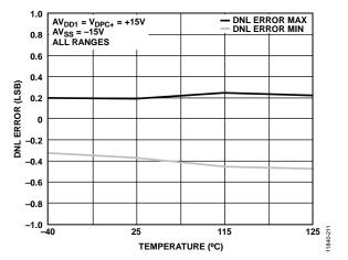
Figure 36. DNL vs. Temperature
