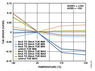
Figure 37. Total Unadjusted Error vs. Temperature, Internal RSET
