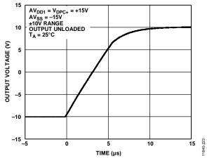
Figure 22. Full-Scale Positive Step
