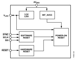
Figure 76. Power-On Reset Block Diagram
