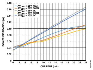
Figure 61. Power Dissipation vs. Current
