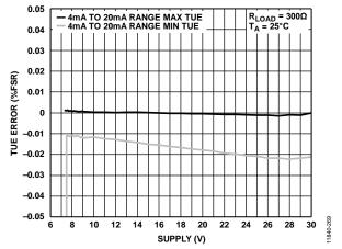
Figure 44. Total Unadjusted Error vs. AV<sub>DD1</sub>/|AV<sub>SS</sub>| Supply, External R<sub>SET</sub>
