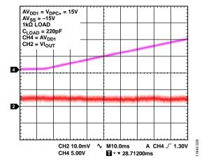
Figure 28. Vout vs. Time on Power Up
