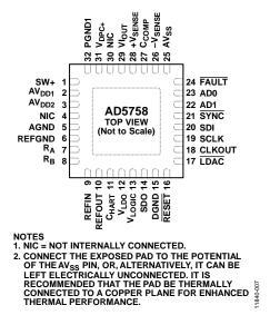
Figure 6. Pin Configuration
