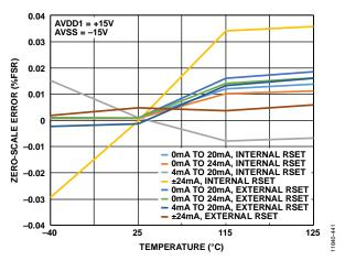
Figure 41. Zero-Scale Error vs. Temperature
