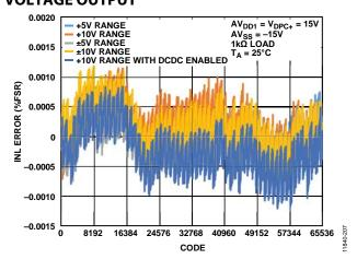
Figure 7. INL Error vs. DAC Code
