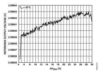
Figure 67. Reference Output Voltage vs.  $AV_{DD2}$  Supply
