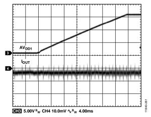
Figure 49. Output Current vs. Time on Power-Up
