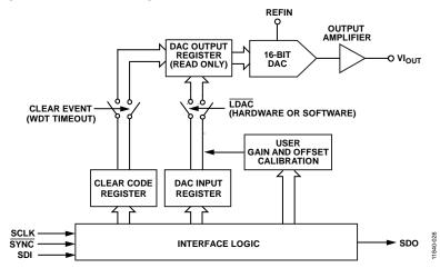
Figure 82. Simplified Serial Interface of Input Loading Circuitry
