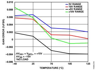
Figure 15. Gain Error vs. Temperature
