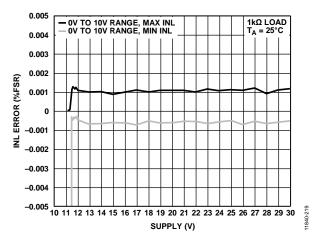
Figure 18. INL Error vs. AVDD1/|AVSS| Supply
