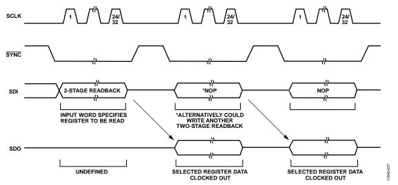
Figure 86. Two Stage Readback Example
