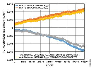
Figure 33. Total Unadjusted Error vs. DAC Code
