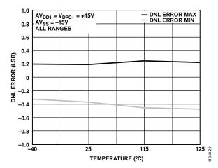
Figure 11. DNL Error vs Temperature
