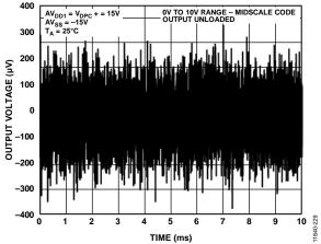
Figure 26. Peak-to-Peak Noise (100 kHz Bandwidth)
