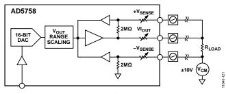
Figure 78. Voltage Output
