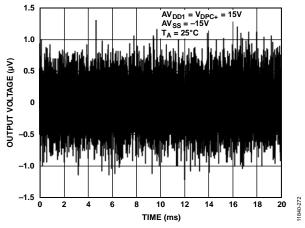
Figure 65. Peak-to-Peak Noise (100 kHz Bandwidth)
