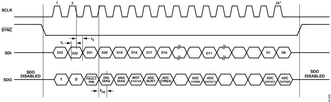
1IF ANY EXTRA SCLK FALLING EDGES ARE RECEIVED AFTER THE 24<sup>TH</sup> (OR 32<sup>ND</sup>, IF CRC IS ENABLED) SCLK, BEFORE SYNC RETURNS HIGH, SDO CLOCKS OUT 0.
