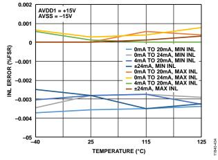
Figure 34. INL Error vs. Temperature, Internal RSET
