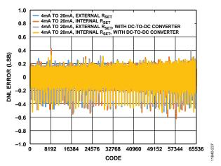
Figure 32. DNL Error vs. DAC Code
