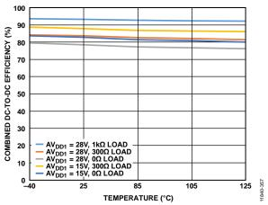
Figure 58. Combined DC-to-DC Efficiency vs. Temperature
