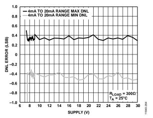
Figure 45. DNL Error vs. AV<sub>DD1</sub>/|AV<sub>SS</sub>| Supply, Internal R<sub>SET</sub>
