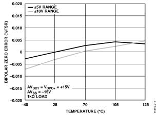
Figure 16. Bipolar Zero Error vs. Temperature
