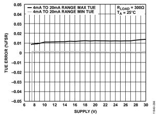
Figure 43. Total Unadjusted Error vs. AV<sub>DD1</sub>/|AV<sub>SS</sub>| Supply, Internal R<sub>SET</sub>
