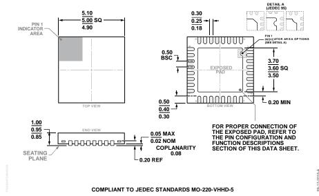
Figure 92. 32-Lead Lead Frame Chip Scale Package [LFCSP] 5 mm × 5 mm Body and 0.95 mm Package Height (CP-32-30) Dimensions shown in millimeters
