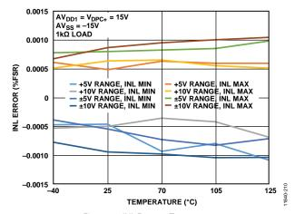
Figure 10. INL Error vs. Temperature
