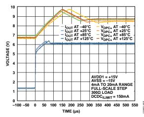
Figure 54. Output Current and V<sub>DPC+</sub> Settling Time vs. Temperature
