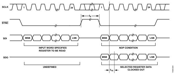
Figure 3. Readback Timing Diagram
