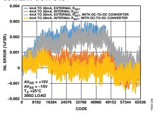
Figure 31. INL Error vs. DAC Code
