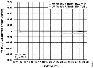
Figure 20. Total Unadjusted Error vs. AV<sub>DD1</sub>/|AV<sub>SS</sub>| Supply
