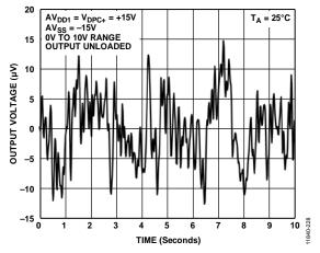
Figure 25. Peak-to-Peak Noise (0.1 Hz to 10 Hz Bandwidth)
