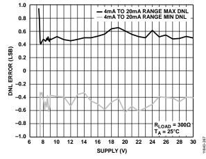
Figure 46. DNL Error vs. AVDD1/AVSS Supply, External RSET
