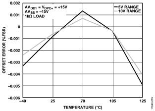
Figure 14. Offset Error vs. Temperature
