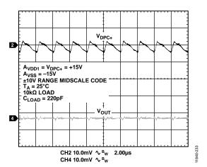
Figure 30. Voltage Output Ripple
