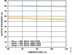
Figure 60. Output Efficiency vs. Temperature
