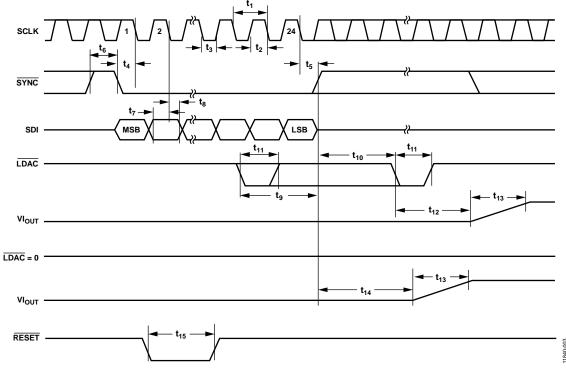
Figure 2. Serial Interface Timing Diagram
