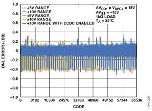
Figure 8. DNL Error vs. DAC Code
