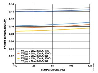
Figure 62. Power Dissipation vs. Temperature
