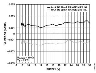
Figure 47. INL Error vs. AV<sub>DD1</sub>/|AV<sub>SS</sub>| Supply, Internal R<sub>SET</sub>
