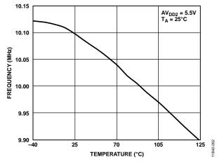
Figure 72. Internal Oscillator Frequency vs. Temperature
