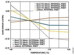
Figure 42. Gain Error vs. Temperature
