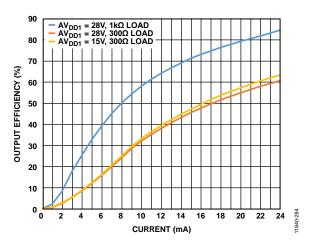
Figure 59. Output Efficiency vs. Current
