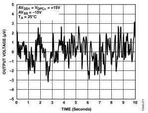
Figure 64. Peak-to-Peak Noise (0.1 Hz to 10 Hz Bandwidth)
