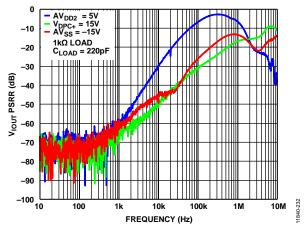
Figure 29. Vout PSRR vs. Frequency
