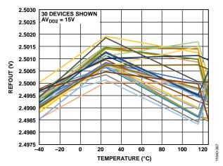
Figure 68. REFOUT vs. Temperature
