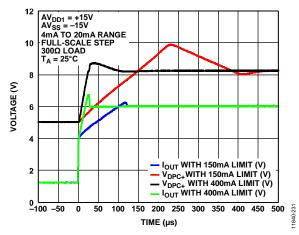
Figure 52. Output Current and  $V_{DPC+}$  Settling Time 300  $\Omega$  Load
