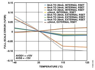
Figure 40. Full-Scale Error vs. Temperature
