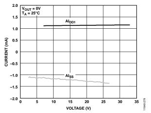
Figure 70. Al<sub>DD1</sub>/Al<sub>SS</sub> Current vs. AV<sub>DD1</sub>/|AV<sub>SS</sub>| Supply
