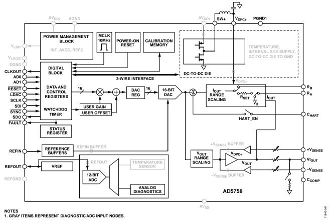
Figure 84. Diagnostic ADC Input Nodes
