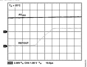
Figure 63. REFOUT Turn On Transient
