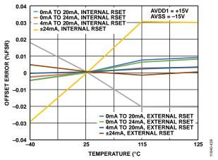
Figure 39. Offset Error vs. Temperature
