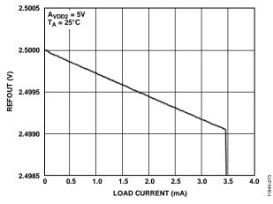
Figure 66. REFOUT vs. Load Current
