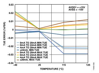
Figure 38. Total Unadjusted Error vs. Temperature, External RSET
