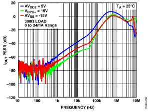
Figure 56. Iouт PSRR vs. Frequency
