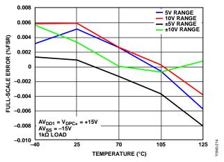
Figure 13. Full-Scale Error vs. Temperature
