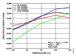
Figure 17. Zero-Scale Error vs. Temperature
