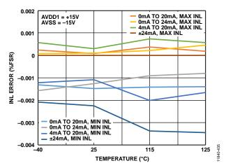
Figure 35. INL Error vs. Temperature, External R<sub>SET</sub>
