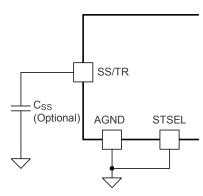
Figure 35. Slow Start Capacitor (C<sub>SS</sub>) and STSEL Connection
