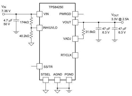
Figure 28. Typical Schematic VIN = 7 V to 36 V, VOUT = 3.3 V
