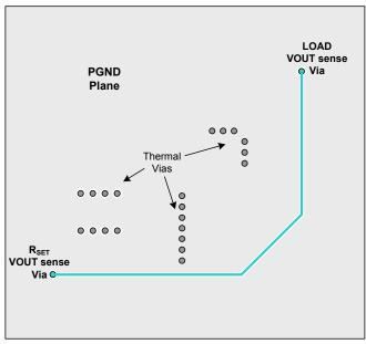
Figure 41. Typical PGND-Layer Recommended Layout
