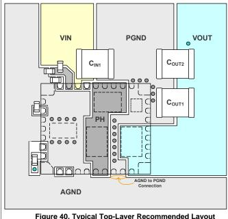
Figure 40. Typical Top-Layer Recommended Layout
