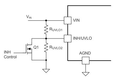
Figure 32. Typical Inhibit Control
