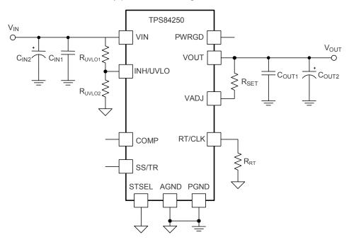
Figure 25. TPS84250 Typical Schematic
