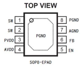
Figure 3. PIN Configuration
