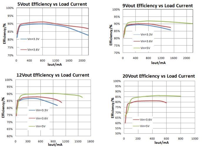
Note: Efficiency data is based on demo test at 20°C. If work at big current for long time, maybe thermal shutdown. its load capacity is related with heat dissipation conditions.
