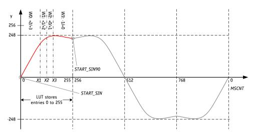
Figure 15.1 LUT programming example
