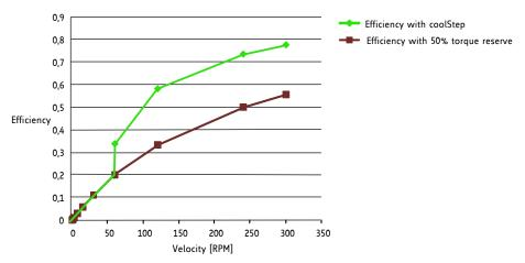
Figure 1.2 Energy efficiency with coolStep (example)
