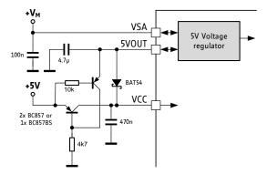
VCC supplied from external 5V. 3.3V IO voltage generated from same source.
