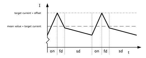
Figure 9.4 Classic const. off time chopper with offset showing coil current
