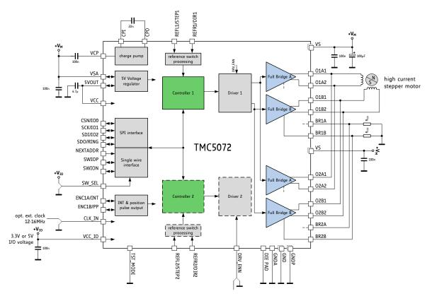
Figure 3.3 Driving a single motor with high current
