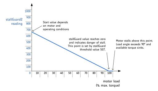
Figure 12.1 Function principle of stallGuard2
