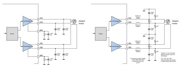
Figure 3.7 Simple ESD enhancement and more elaborate motor output protection
