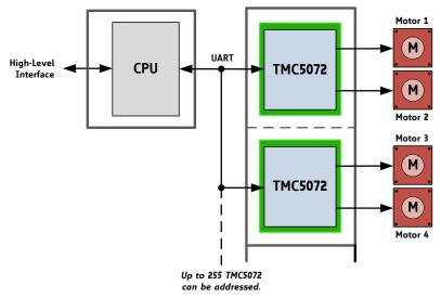
An application for up to 510 stepper motors is shown. The UART single wire differential interface allows for a decentralized distributed system with a minimized number of components. Additionally, ABN an encoder and up to two reference switches can be used for each motor. A single CPU can control the whole system. The CPUboard and controller / driver boards are highly economical and space saving.
