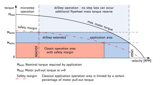
Figure 14.1 dcStep extended application operation area
