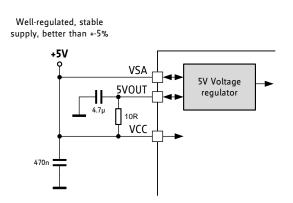
Figure 3.5 Using an external 5V supply to bypass internal regulator
