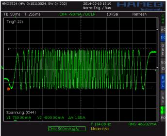
Figure 8.2 Scope shot: good setting for PWM\_GRAD
