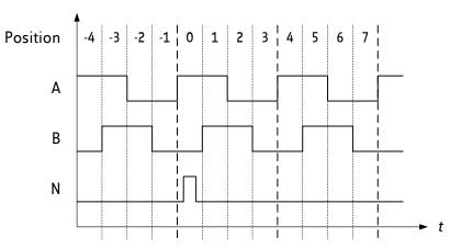
Figure 17.1 Outline of ABN signals of an incremental encoder
