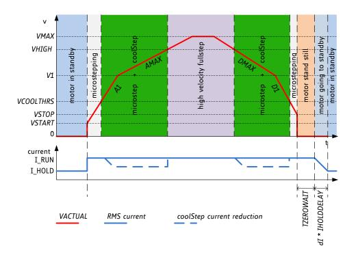
Figure 11.3 Ramp generator velocity dependent motor control
