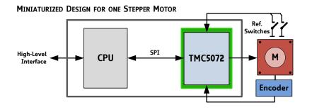
The stepper motor driver outputs are switched in parallel. A dual ABN encoder interface and two reference switch inputs are used.
