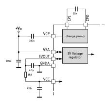
Figure 3.6 RC-Filter on VCC for reduced ripple
