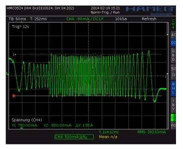
Figure 8.3 Scope shot: too small setting for PWM\_GRAD
