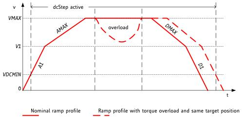
Figure 14.2 Velocity profile with impact by overload situation
