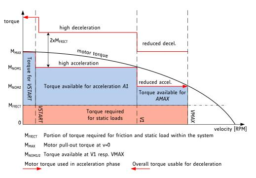
Figure 11.2 Illustration of optimized motor torque usage with TMC5072 ramp generator
