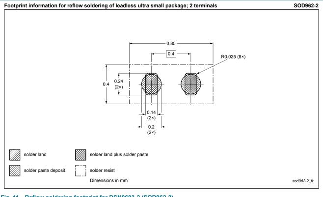
Fig. 11. Reflow soldering footprint for DSN0603-2 (SOD962-2)
