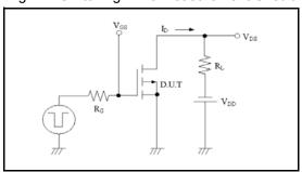
Fig.2-1 Gate Charge Measurement Circuit
