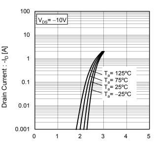
Gate - Source Voltage : -V<sub>GS</sub> [V]
