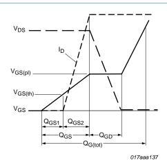
Fig 15. Gate charge waveform definitions
