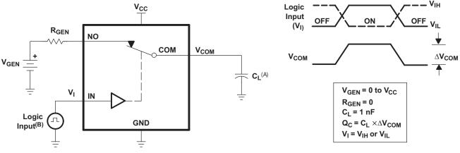
A. C<sub>L</sub> includes probe and jig capacitance.
