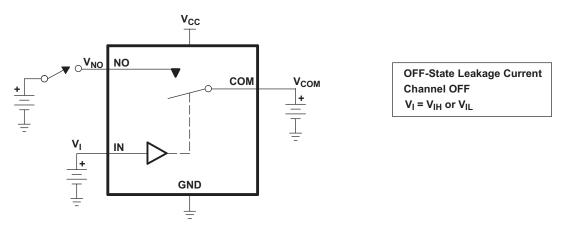
Figure 16. OFF-State Leakage Current (I<sub>COM(OFF)</sub>, I<sub>NO(OFF)</sub>, I<sub>COM(PWROFF)</sub>, I<sub>NOC(PWR(FF)</sub>)
