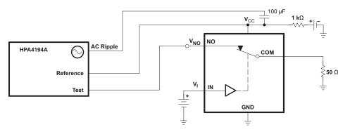
Figure 25. Power Supply Rejection Ratio (PSRR)
