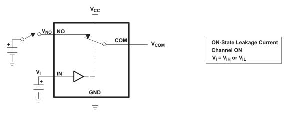
Figure 17. ON-State Leakage Current (I<sub>COM(ON)</sub>, I<sub>NO(ON)</sub>)
