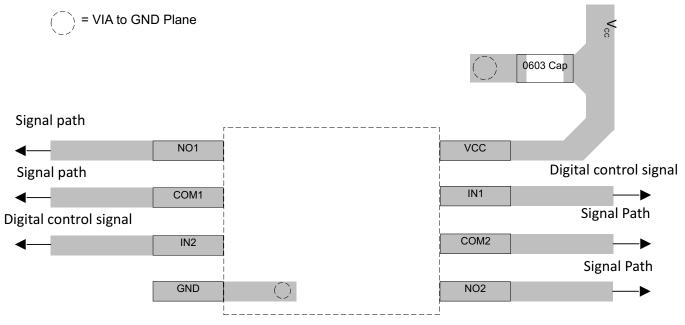
Figure 28. TS5A21366 Layout Example
