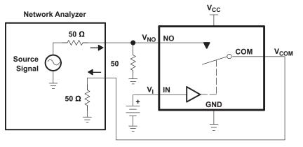
Figure 21. OFF Isolation (O<sub>ISO</sub>)
