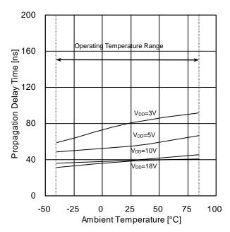
Figure 15. Propagation Delay Time CONT→OUT(t<sub>PHZ</sub>) vs Ambient Temperature
