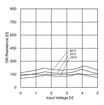
Figure 9. ON Resistance vs Input Voltage (V<sub>DD</sub>=5V, V<sub>EE</sub>=0V, CONT=5V)
