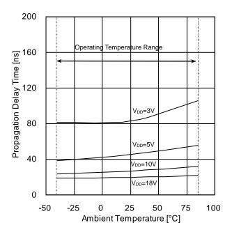
Figure 17. Propagation Delay Time CONT→OUT(t<sub>PZL</sub>) vs Ambient Temperature
