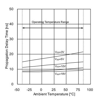
Figure 13. Propagation Delay Time IN→OUT(t<sub>PHL</sub>) vs Ambient Temperature
