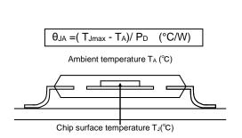
Figure 18. Thermal Resistance
