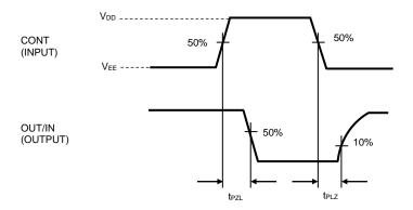
Figure 5. Propagation Delay Time CONT→OUT (t<sub>PZL</sub>,t<sub>PLZ</sub>) Input/Output Waveform
