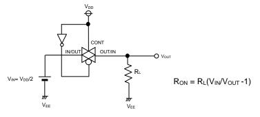
Figure 7. ON Resistance (RoN) Test Circuit
