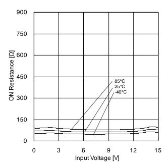
Figure 11. ON Resistance vs Input Voltage (V<sub>DD</sub>=15V, V<sub>EE</sub>=0V, CONT=15V)
