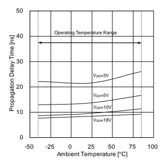
Figure 12. Propagation Delay Time IN→OUT(t<sub>PLH</sub>) vs
