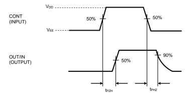
Figure 3. Propagation Delay Time CONT→OUT (t<sub>PZH</sub>,t<sub>PHZ</sub>) Input/Output Waveform
