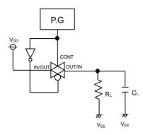
Figure 4. Propagation Delay Time CONT→OUT (tpzH,tpHz) Test Circuit
