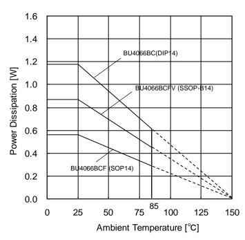
Figure 19. Derating Curve
