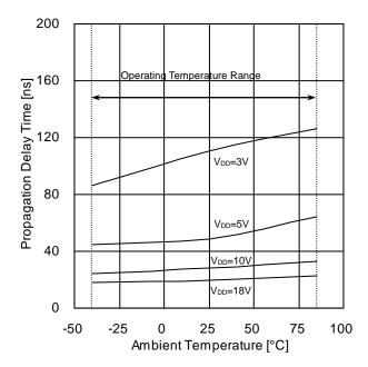
Figure 14. Propagation Delay Time CONT→OUT(t<sub>PZH</sub>) vs Ambient Temperature
