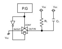
Figure 6. Propagation Delay Time CONT→OUT (tpzL,tplz)
