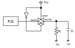
Figure 1. Propagation Delay Time IN→OUT(t<sub>PHZ</sub>,t<sub>PLZ</sub>)
