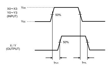
Figure 1. Propagation Delay Time (IN→OUT) (t<sub>PLH</sub>,t<sub>PHL</sub>)
