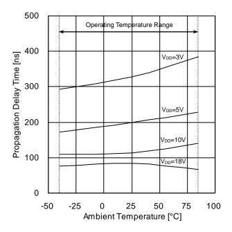
Figure 15. Propagation Delay Time  $t_{PLZ}$  (CONTROL (A,B) $\rightarrow$ OUT) vs Ambient Temperature
