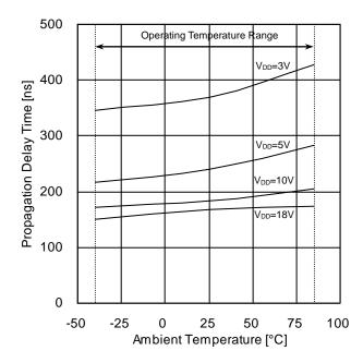
Figure 13. Propagation Delay Time t<sub>PZH</sub> (CONTROL (A,B)→OUT) vs Ambient Temperature
