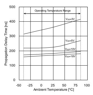
Figure 18. Propagation Delay Time t<sub>PHZ</sub> (CONTROL (INHIBIT)→OUT) vs Ambient Temperature
