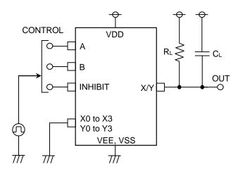
Figure 6. Test Circuit 3 (tpzL,tpLz)
