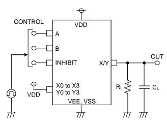
Figure 4. Test Circuit 2 (tpzh,tphz)
