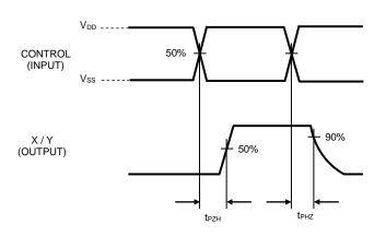
Figure 3. Propagation Delay Time (CONTROL (A,B,INHIBIT) $\rightarrow$ OUT) ( $t_{PLH},t_{PHL}$ )
