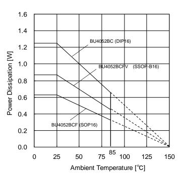
Figure 22. Derating Curve
