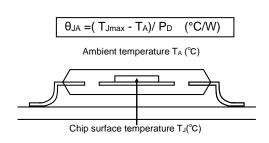
Figure 21. Thermal Resistance
