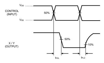
Figure 5. Propagation Delay Time (CONTROL (A,B,INHIBIT) $\rightarrow$ OUT) (tpzL,tpLZ)
