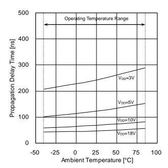
Figure 19. Propagation Delay Time  $t_{PZL}$  (CONTROL (INHIBIT) $\rightarrow$ OUT) vs Ambient Temperature
