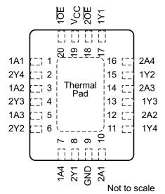
Figure 5-4. RWP Package 20-Pin X1QFN Top View
