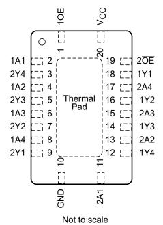
Figure 5-3. RGY Package 20-Pin VQFN Top View
