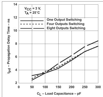
Figure 6-1. Propagation Delay (Low to High Transition)
