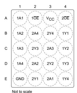
Figure 5-1. ZQN Package 20-Pin BGA Top View
