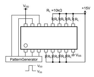
Figure 6. Test Circuit of Timing Characteristics
