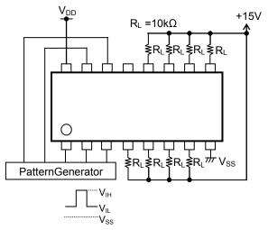
Figure 2. Test Circuit of Input H/LVoltage
