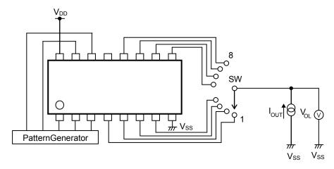
Figure 3. Test Circuit of Output L Voltage
