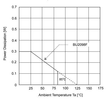
Figure 8. Derating Curve
