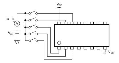
Figure 4. Test Circuit of Input H/LCurrent
