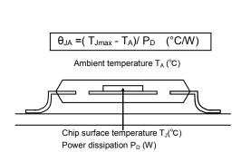
Figure 7. Thermal resistance
